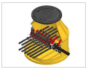
HIRO Manifold Chambers M provide security as well as a central location for controlling and monitoring the flow and pressure of up to 12 brine circuits and are typically used for large domestic geothermal ground source heat recovery systems.
